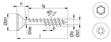
Tip: sharp, Type 17, Saw Thread and Type 17 & Saw Thread combined Shank Rips: optional for L >=25mm and d >=3,5; obligatory for L >=220mm Under Head Rips or Pockets: optional Thread Cutting Line: optional Head Mark: optional
