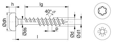
Tip: sharp, Type 17, Saw Thread and Type 17 & Saw Thread combined Shank Rips: optional for L >=25mm and d >=3,5; obligatory for L >=220mm Thread Cutting Line: optional Head Mark: optional
